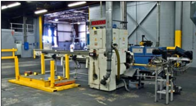
Figure 5. One of IEI's nine Kasto precision saws, capable of producing very tight tolerance lengths.
