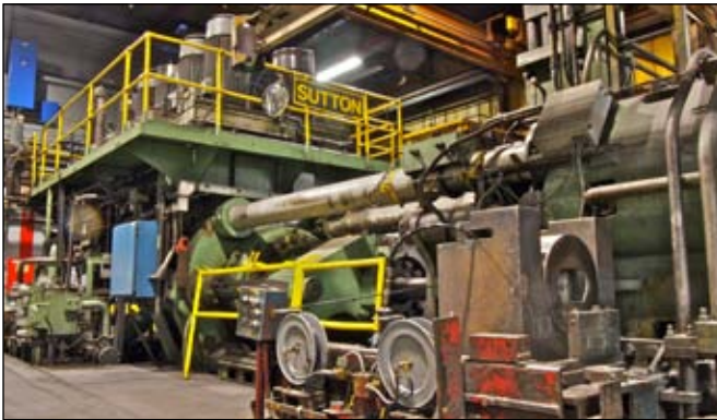
Figure 4. The 3,300 ton 10" Sutton extrusion press.
